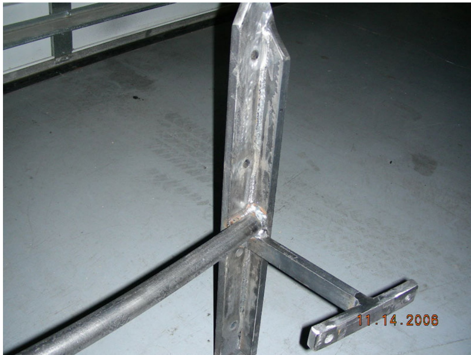
Rear view of Passenger side. Note solid round stock welded on TOP of bumper support bracket. Angle of bumper mounts must be matched to YOUR exact vehicle.
