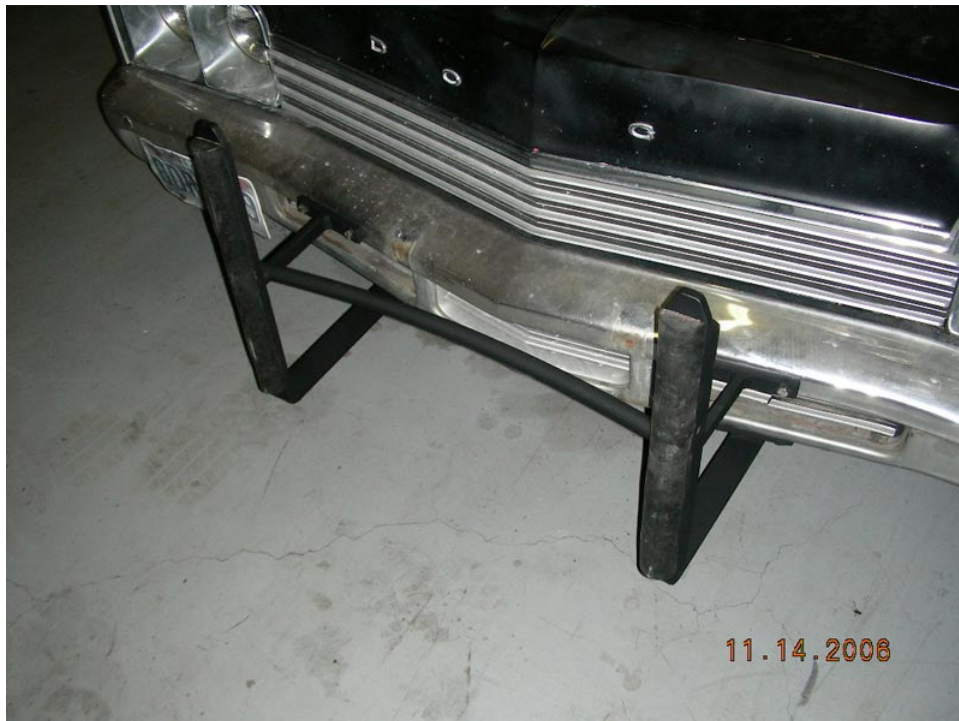
View from drivers side. Note bend in round bar.
