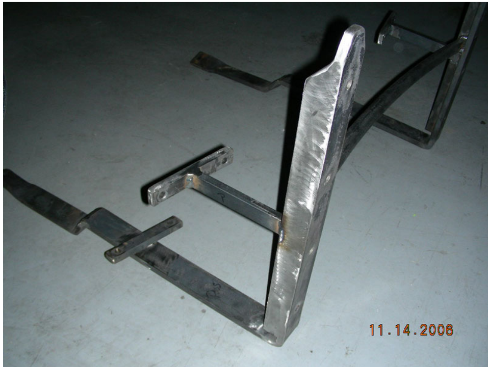
Side \frac{3}{4} View. Viewed from passenger side. Note weld joint has been ground smooth. Also \frac{1}{2} " gap between lower support and side support.
