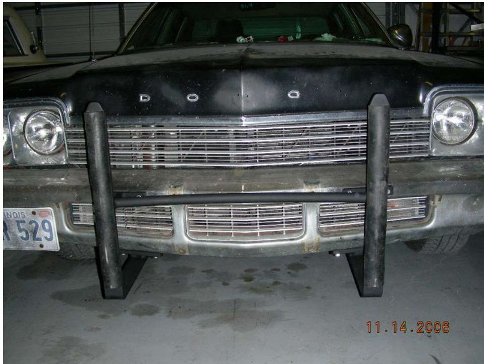
Centered on car. Tips of pushbar BELOW hood line. Note: pushbar rubber mounted 1" below top of pushbars.
